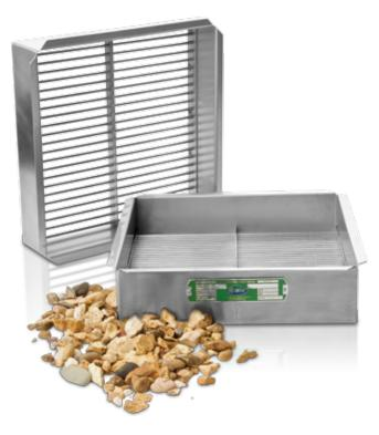
Used to determine the flakiness index of aggregates. Endecotts grid sieves are manufactured to fully conform to the requirements of EN 933-3:1997. The  $300 \times 300$  mm sieves are made entirely of stainless steel and are strong, durable and anti-corrosive. They can be supplied as a single item or as a set of 13 sieves.
